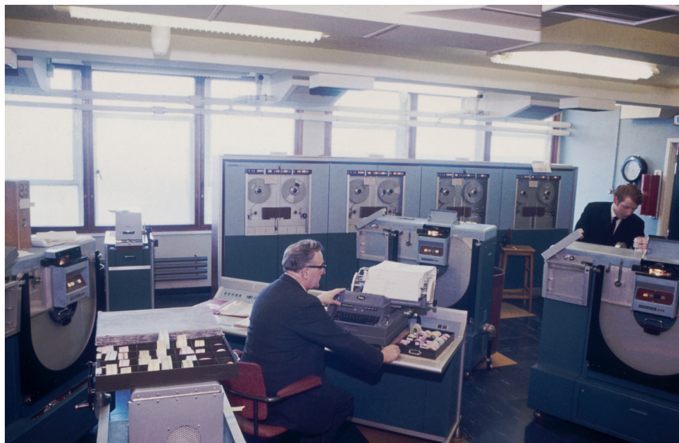
Fig. 1. The Met Office computer, console operator's desk. KDF-9 tape unit behind, Met Office Headquarters, Bracknell. Scanned from the original 35 mm slide, image no. 2306, item ID 962305-1001. ©Crown copyright.
